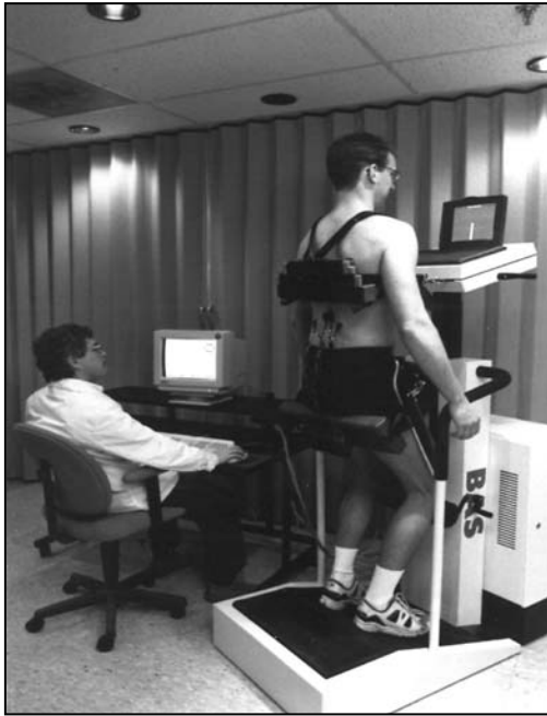
Figure 1. A subject is shown being tested in the Back Analysis System (BAS). The subject's task is to try and extend their trunk against the Data from SEMG electrodes and load cells are acquired and processed from the desktop PC.
